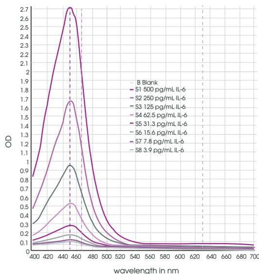
**Figure 2. Representative spectral data.** Spectral data collected on samples containing the indicated concentrations of IL-6. Selection of peak (450 nm) off-peak (466 nm) and reference (630 nm) wavelengths are indicated by dashed lines.
